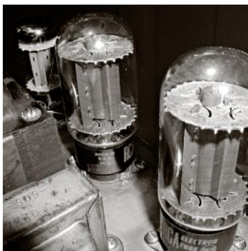
It's *always* necessary to check tube bias on any amp even if there is no adjustment when tubes are replaced. All tubes are uniquely variable, so idle currents for any specific tube will vary from tube to tube, even in matched sets. Some folks think that you can simply plug in a set of
