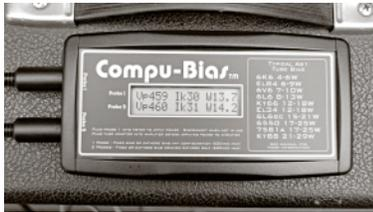
Also, all of the voltages that come from the probe to the Compu-Bias are *low level*, with no high voltages going to the meter. This a serious
